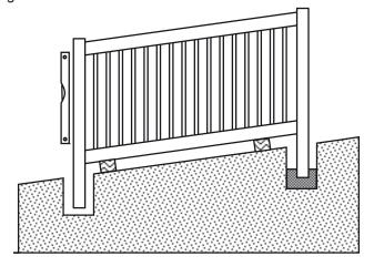
Step 3 - Install second panel as above, butting the posts together. Fasten with 3 self tapping screws as shown. These are self drilling and self tapping and require only a screwdriver tip in an electric drill with a Phillips no. 2 head to screw them in. Partially fill second hole and tamp down as before
