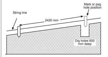
Step 2 - Install the first panel using props or chocks to position the panell. To rack the panel and bring the bottom rail parallel to the ground simply brace the opposite corner against a firm object and lightly tap the corner. Partially fill the first hole with dry concrete mix and tamp down to hold bottom of the post in position. To comply with pool fencing regulations, ensure the gap under the bottom rail is less than 100mm and the top rail is at least 1.2m above the ground
