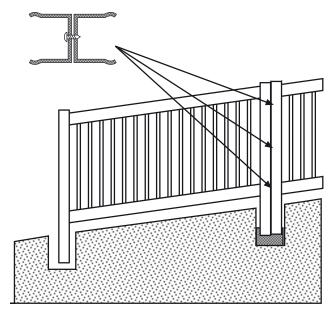
Step 4 - Repeat step 3 with each panel until the end of the run, then sight along the fence for straightness and view from the front to ensure the fence follows the requried contour. Avoid having the fence zig zag up and down. Fill each hole with wet concrete noting that the concrete must be level with or slightly above the soil. Slope the top of the concrete to allow water to run off.
